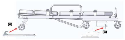
2) Do it a mark on the both sides the drill positions on the vehicle floor, (A) and (B). The necessary holes for each side are indicated with red arrows. Leave a minimum space of 12cm between the cot and the ambulance wall / furniture, allowing free movement (turning) of the stretcher wheels (C).
