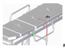
3) Backrest system: Press the lever (A), raising or lowering the backrest at the desired angle (B), releasing the lever and allowing it to lock automatically in one of the height positions.
