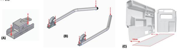
ATTENTION: The fasten rail has several sequential holes. Choose the best drilling position according to the characteristics and availability of the floor of your ambulance.
