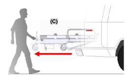
ATTENTION: Be careful when the ambulance is parked on steep or uneven terrain. Tilt of the cot may be necessary to compensate for leveling and full opening of the articulation set. When pulling the cot out of the ambulance, release the retract lever and check that the articulation set has been correctly armed.
