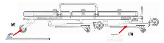
2) Do it a mark on the both sides the drill positions on the vehicle floor, (A) and (B). The necessary holes for each side are indicated with red arrows. Leave a minimum space of 12cm between the cot and the ambulance wall / furniture, allowing free movement (turning) of the stretcher wheels (C).
