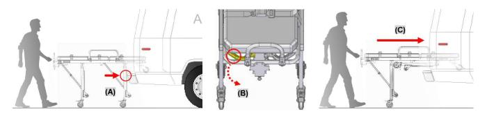
2) Loading the cot by releasing the retraction lever until the rear legs are evenly touching the ambulance bumper (D). After touching the rear legs against the ambulance bumper, pull the right retraction lever (E), loading the cot completely into the ambulance until it locks on the fastening system (F).
