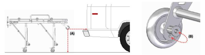
ATTENTION: Cots with different height levels from the ambulance floor have a great risk of falling when unloading from the ambulance. If the cot has a different height level between the loading wheels and the ambulance floor, keep it out of the service until to height adjust can be made according to the prior instructions.
