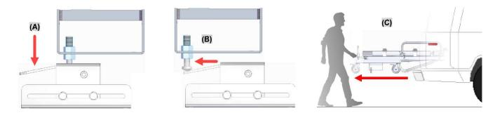
ATTENTION: Be careful when the ambulance is parked on steep or uneven terrain. Tilt of the cot may be necessary to compensate for leveling and full opening of the articulation set. When pulling the cot out of the ambulance, release the retract lever and check that the articulation set has been correctly armed.
